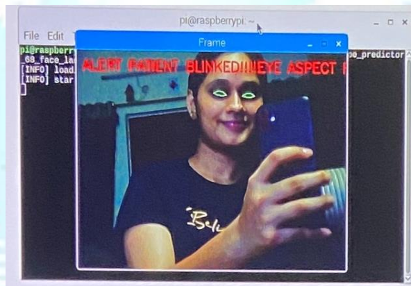
Figure 9: EAR is high because the eyes were opened — the patient has blinked.
